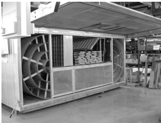
Figure 1: Laboratory kiln drier to be used for the experiments
