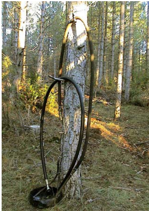
Used oily hoses draining into a recipient before removal to a collection point. Waste specific to harvesters and forwarders.
