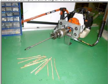
Drill. It is a non-destructive method for trees. Collected chips may serve to measure the tree fibres morphology.
