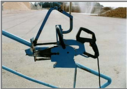
Chain saw. Sample may be a roundwood taken on a log and used for fibre morphology analyses, or sawdust collected during sawing
