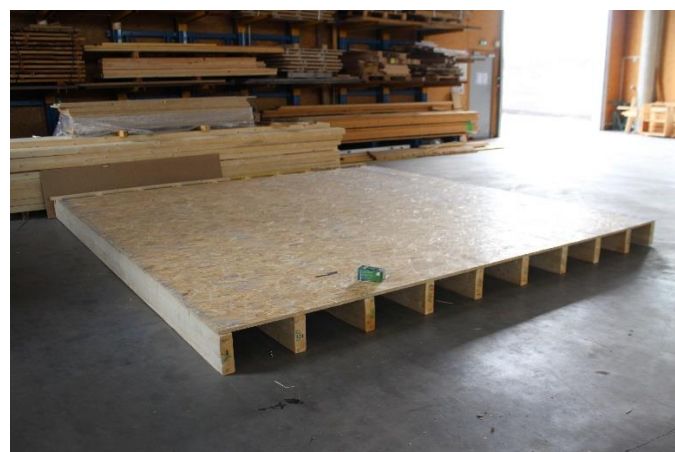
Figure 1 - Plancher solives-OSB testé
